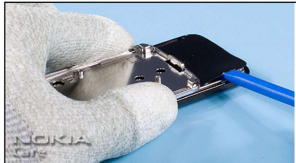
20. Partly lift up the glued in BACK PLATE with the SS-93.
